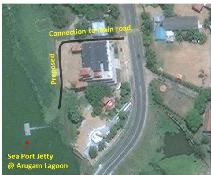
Figure 40: The proposed two access ways connecting the floating plane pier with the Pottuvil – Panama road
